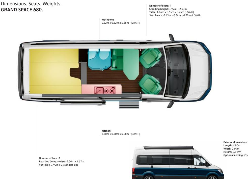
Length: 6.80m Width: 2.04m Height: 2.84m<sup>1</sup> Optional awning: 2.50m x 3.50m (L/W)
