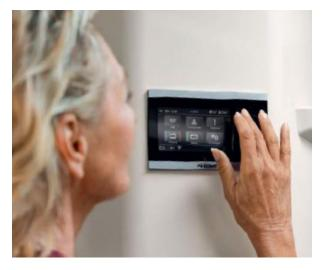
**01 Central operating unit with touch pad for monitoring and controlling the heater, water supply and batteries.** A convenient way to adjust and control everything that makes modern camping so great.
