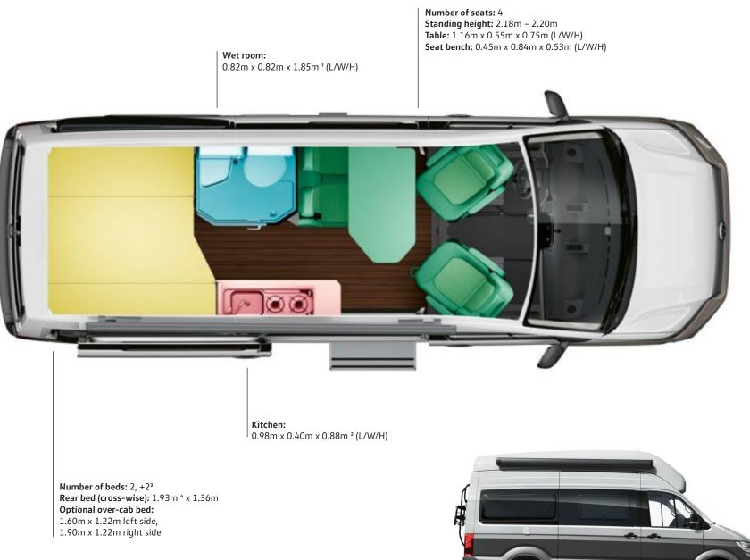
Exterior dimensions: Length: 5.98m Width: 2.04m <sup>5</sup> Height: 2.97m <sup>6</sup> Optional awning: 2.50m x 3.00m (L/W)
