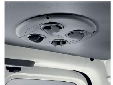
Optional load compartment ventilation.
