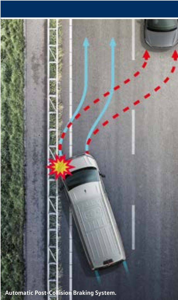
(MCB) Automatic Post-Collision Braking System. Fitted as standard, the Automatic Post-Collision Braking System triggers braking after a collision, with the aim of preventing secondary collisions.
