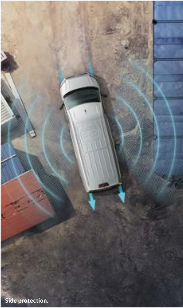
P Side protection. Available as an option, Side protection monitors the vehicle's sides and alerts you with visual and audible warnings if you're getting too close to other vehicles, pillars, walls or pedestrians.
