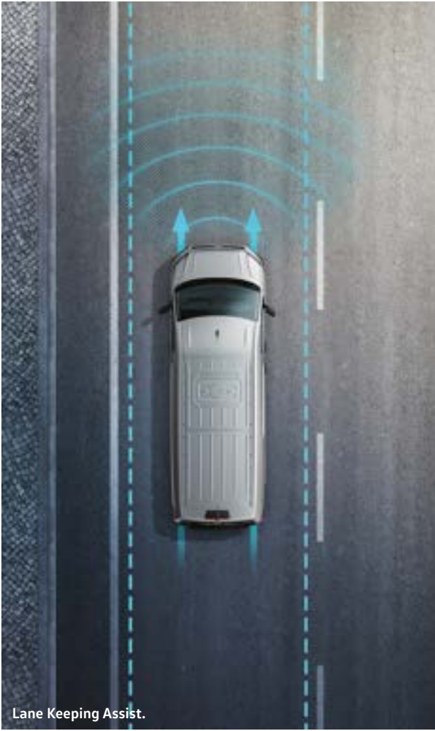
Lane Keeping Assist. Available as an option, Lane Keeping Assist countersteers the vehicle if the driver unintentionally drifts from a lane. The system also emits audible and visual warnings via the multi-function display to alert the driver of danger.
