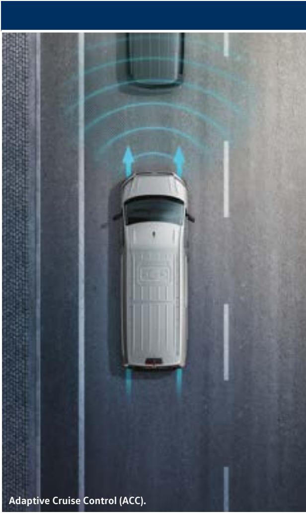
Adaptive Cruise Control (ACC) (optional) Available as an option on Commerce Plus only, ACC uses a front radar to measure the distance (up to 120 metres) and speed relative to vehicles driving ahead. It automatically regulates the pre-set distance. ACC also includes the Front Assist with City Emergency Braking System. This detects critical distances, warns of hazardous situations and when necessary, a speed of up to 18mph triggers emergency braking.
