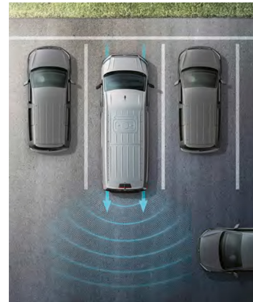
Parking assistant (schematic representation using the example Crafter model).
