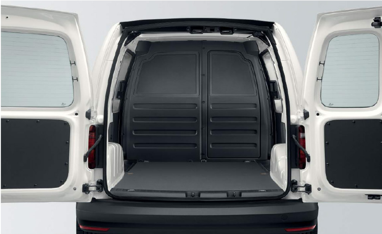
Full-height solid bulkhead. Standard on Caddy Maxi panel van.
