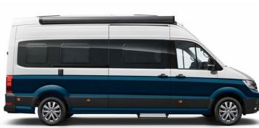
Exterior dimensions: Length: 6.80m Width: 2.04m Height: 2.84m<sup>1</sup>
